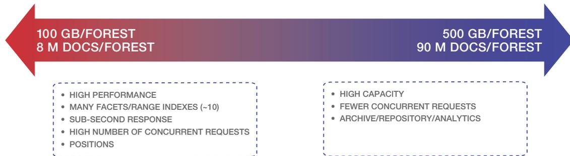
Figure 4: Forest sizes for high performance and high capacity applications
